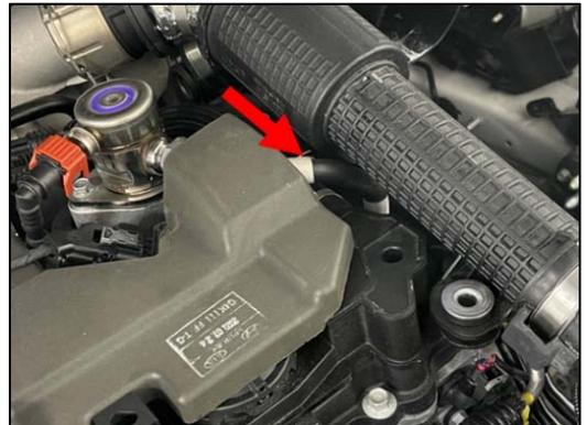
3. On the high-pressure fuel pipe insulator, locate the printed LOT number.
